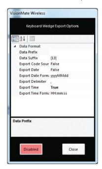
the keyboard wedge export. The button on the left, colored red, allows you to enable or disable automatic code export via keyboard wedge.
