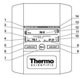
Figure. 33. iCan™ touchscreen with combined gas connection
