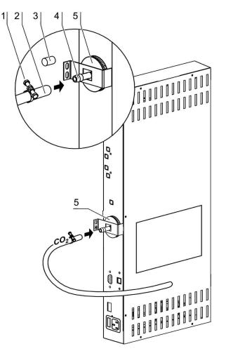
Figure. 24. Installing gas pressure hoses
