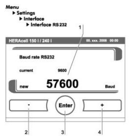
Figure. 45. RS 232 interface baud rate setting
