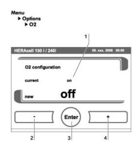
Figure. 58. Switching the  $O_2$  control on and off
