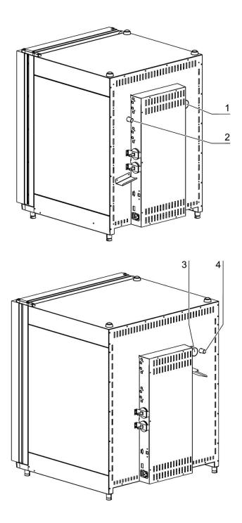
Figure. 15. Rear panel openings
