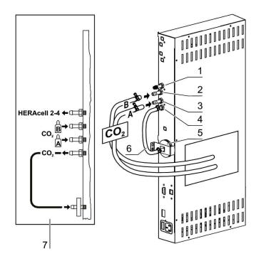
Figure. 26. Gas connection with gas monitoring system (optional)
