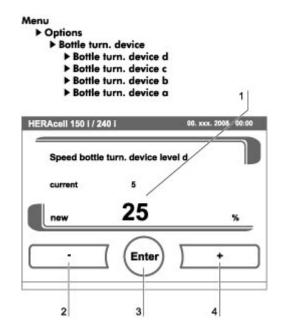
Figure. 57. Bottle turning device speed setting
