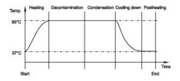
Figure. 66. Decontamination routine phases
