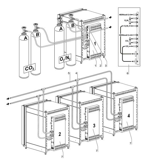
Figure. 6. Looped-through gas supply HERACELL® 150i
