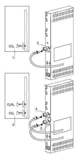
Figure. 25. Gas connection without gas monitoring system
