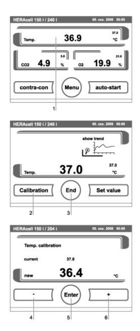
Figure. 71. Temperature calibration procedure
