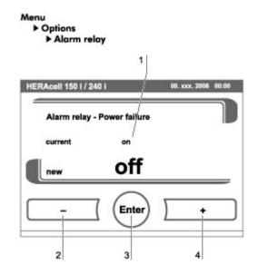
Figure. 52. Alarm relay setting
