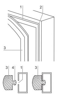
Figure. 77. Magnetic door seal replacement
