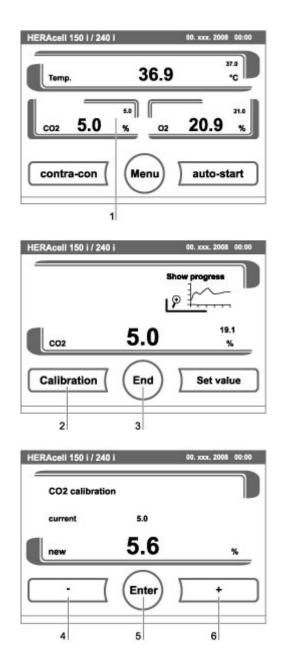
Figure. 74.  $CO_2$  calibration procedure
