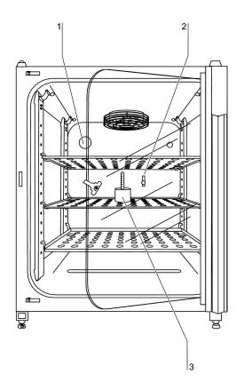
Figure. 70. Preparing the temperature calibration
