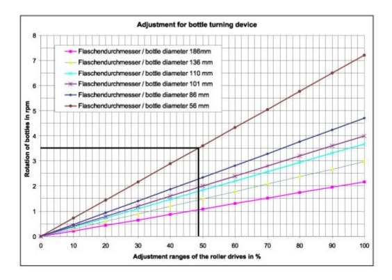
Figure. 22. Bottle turning speed
