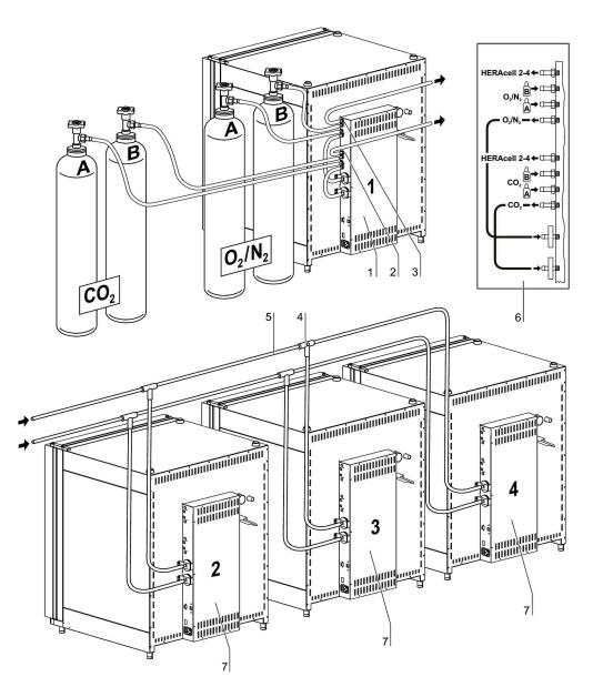
Figure. 9. Looped-through gas supply HERACELL® 240i
