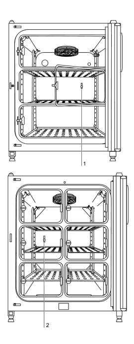
Figure. 73. Gas-tight screen measurement opening
