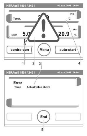
Figure. 65. Event error overtemperature
