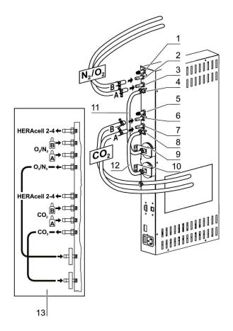
Figure. 27. Combined connection with gas monitoring system (optional)
