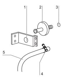
Figure. 75. Gas inlet filter installation
