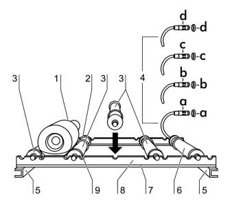
Figure. 21. Installing the bottle turning devices
