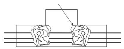
Insert fiber rope material down into horizontal conduit opening. Pressing down firmly, work the material
