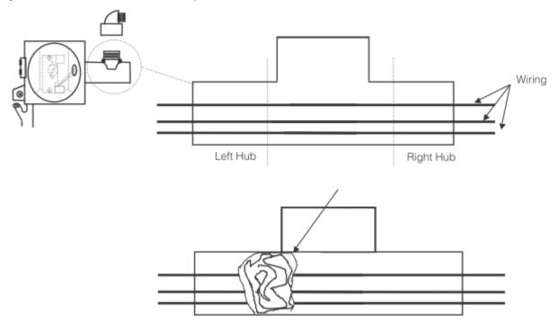
Insert fiber rope material down into horizontal conduit opening. Pressing down firmly, work the
