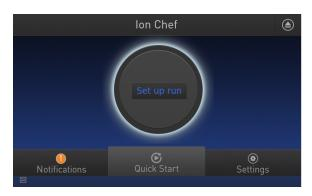
**3.** Touch **Step by Step** to have the instrument lead you through the instrument setup, or touch **Quick Start** to skip the instrument setup screens.
