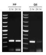
Figure 4. Reaction stability on the benchtop. Assembled PCR reactions were loaded immediately (0 hr) onto a thermal cycler or incubated at room temperature for 24 hours before thermal cycling. With a stringent hot start, of Phusion Plus DNA Polymerase (PP) produced PCR amplicons with high specificity and yields even after 24 hours, in contrast to NEB Q5™ Hot Start High-Fidelity DNA Polymerase (Q5).
