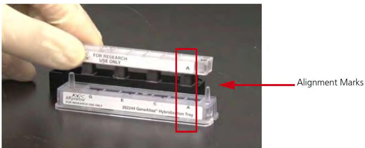
Figure 7 Placing the array strip into the hybridization tray.
