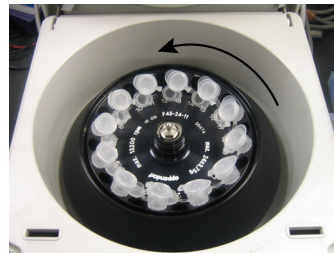
Correct position of tube caps
