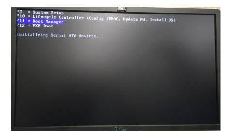
**3.** When the Dell<sup>™</sup> Boot Manager is displayed, use the arrow keys on the keyboard to select **One-shot BIOS Boot Menu**, then press **Enter** on the keyboard.
