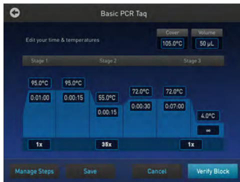
Figure 32 ProFlex™ Thermal Cycler Run Method preview screen
