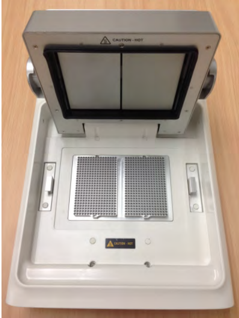
Figure 44 Location of the safety label on the ProFlex™ Dual 384-Well Sample Block
