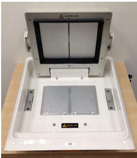
Figure 43 Location of the safety label on the ProFlex™ Dual Flat Sample Block
