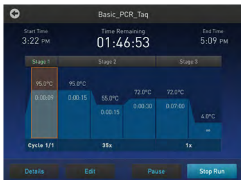
Figure 37 ProFlex™ Thermal Cycler Run Monitoring screen
