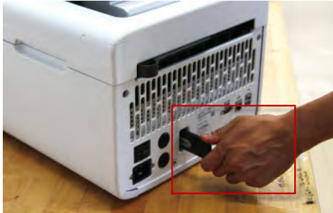
Figure 9 USB port in the ProFlex™ Thermal Cycler unit
