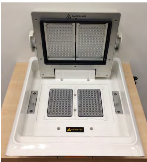
Figure 42 Location of the safety label on the ProFlex™ Dual 96-Well Sample Block
