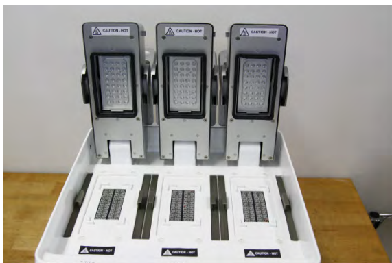
Figure 40 Location of the safety label on the ProFlex™ Thermal Cycler 3x32-Well Sample Block
