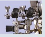
Resterilizable addition valve array facilitates making sterile additions; each vessel can accommodate up to four addition ports; one addition port shown
