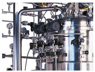
Resterilizable SIP, CIP and addition valves enable sterile transfer of liquids into the vessel for pH and foam control, or nutrient addition
