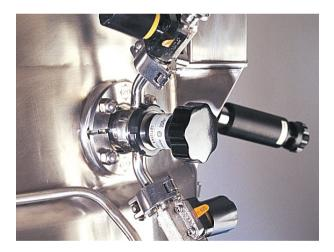
Flush mount, sanitary NA-Connect<sup>®</sup> quick connections in hard-to-clean locations eliminate dead legs; 25 mm safety ports on lower side wall enable use of redundant sensors or retractable housings
