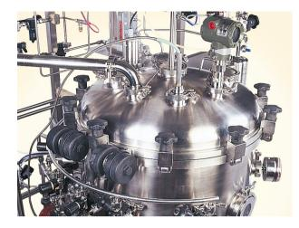
Headplate ports accommodate septum, sprayballs, level sensors, level and pressure transmitters, vessel light and more; spring-assisted manway on 120 - 400 L models; motorized headlift on 1200 L vessel
