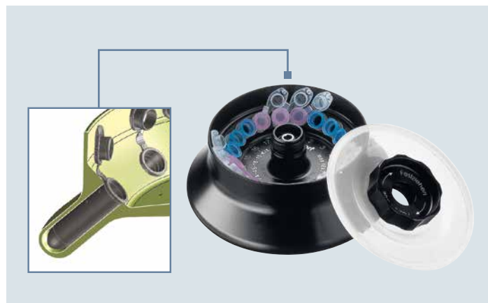
Eppendorf Kit rotor for 18 × spin columns and 1.5/2.0 mL tubes with speed up to 18,111 × g /15,000 rpm. This rotor is designed with an extended rim that protects tube caps from shearing off (FA-45-18-11-Kit; Order no. 5424 706.002).
