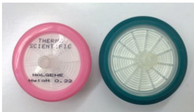
Figure 1. Nalgene syringe filters are smaller than competitors' filters. Nalgene 25 mm filters (left) compared to (A) Pall™ 25 mm and 32 mm filters and (B) Millipore™ 33 mm filters.
