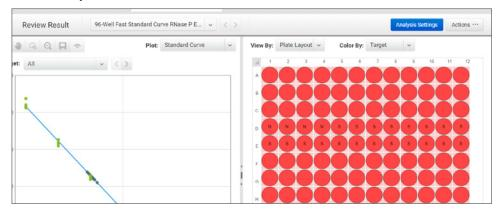
Figure 2. Absolute quantification module for gene expression analysis. The module enables analysis of genes of interest with the use of a standard curve. Additional flexibility is achieved by importing standard curves from other experiments.
