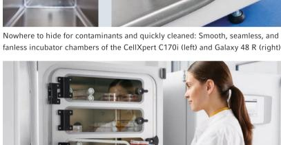
Available with small segmented inner doors to minimize hypoxia disturbance (CellXpert C170i shown here)
