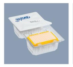
$300 \ \mu L$  tips as reload system (color coded for easy volume identification)
