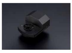
Motorized Attenuator Wheel/U-AW The Olympus BX63 has a motorized ND filter wheel for fluorescence and transmitted light intensity adjustments. \* Special adapters are required for mounting (U-LHEAD for fluorescence, and U-LH100ADP for transmitted light).
