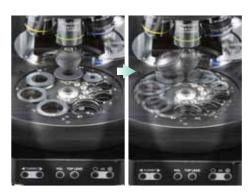
Condenser Design to Reduce Back-reflections The motorized universal condenser is designed to reduce back-reflections and autofluorescence by swinging its top lens out, automatically closing its diaphragm to the minimum, and locating the wheel in between two positions.
