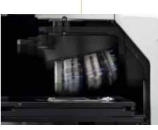
Microscope Frame Equipped with Motorized Focus and Field Diaphragm This unit incorporates a high-speed, highprecision motorized focusing nosepiece with 0.1 µm resolution and 20 mm vertical strokes. The field diaphragm adjustment of transmitted light is also motorized.
