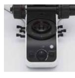
Further Ease in Imaging with Multi-stained Specimens The 8-position fluorescence illuminator allows flexible responses to various fluorescence specimens. Mirror units can easily be replaced.
