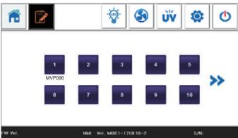
(2) Select desired procedure by press on the touch screen to edit, or create blank procedure.
