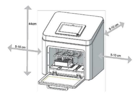
The space for the allocation of SYNC Nucleic Acids Extraction System must secure 5-10 cm distance from the instrument to the wall.
