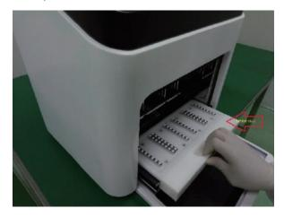
(5) Set up the Magnet sleeve on the mixing sleeve track.
