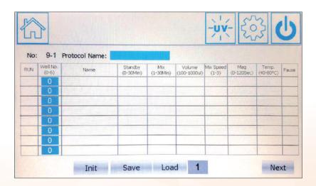
(3) Save a protocol, after enter the desired procedures, make sure the protocol number is not duplicated, and press<Save> to save the protocol.
