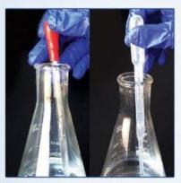
Replaces rubber bulbs and glass pipets, reducing the likelihood of contamination
