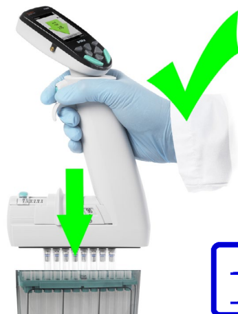
Picture B6. Attachment of 96-format tips
