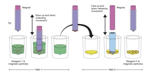
Figure 7. A concentration step during magnetic particle processing
