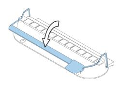
Figure 43. Closing the elution strip holder
