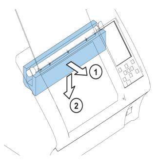
Figure 10. Removing the UV lamp protection
