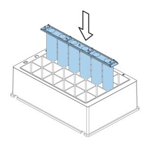
Figure 39. KingFisher Duo Prime 6-tip comb inserted
