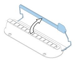
Figure 42. Releasing the elution strip holder
