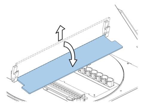
Figure 14. Opening the maintenance door
