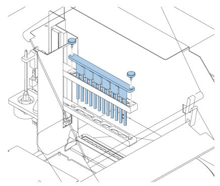
Figure 15. Inserting the KingFisher Duo Prime head
