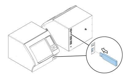
Figure 28. Plugging USB memory device
