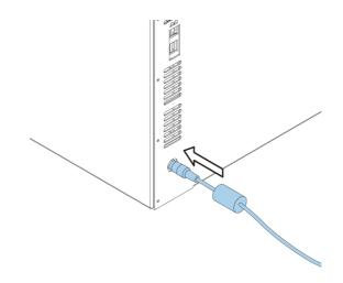
Figure 12. Mains supply cable connected
