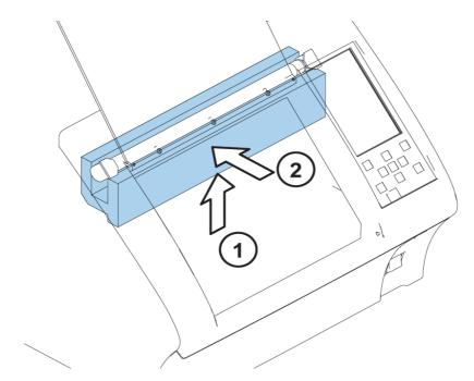
Figure 47. Placing the UV lamp protection
