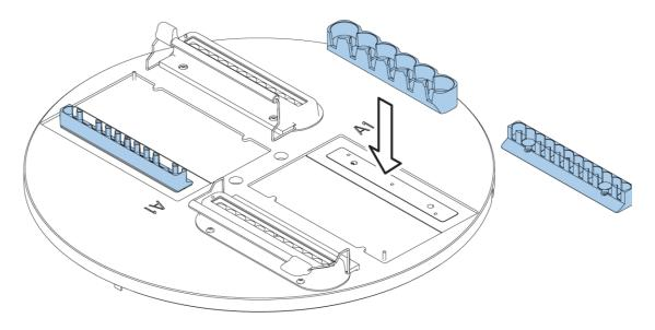
Figure 13. Changing the heating block
