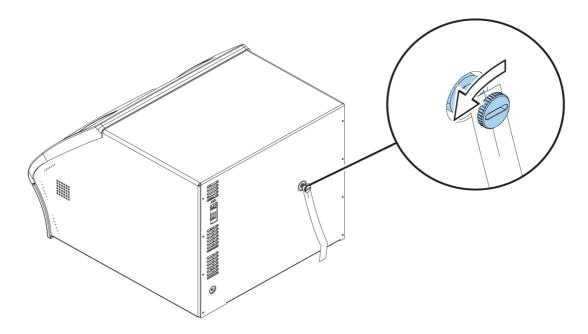
Figure 11. KingFisher Duo Prime transport lock fitted
