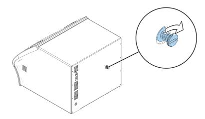
Figure 46. Refitting the transport lock
