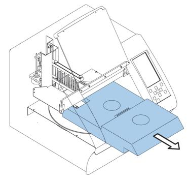
Figure 9. Removing internal cushions
