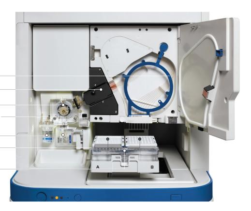
methodologies. The 36 cm and 50 cm arrays have been optimized for many applications for use with POP-7<sup>™</sup> Polymer, POP-6<sup>™</sup> Polymer, and POP-4<sup>™</sup> Polymer run modules. This provides users with flexibility to select their ideal run times and read length needs. The 3500 and 3500xL capillary arrays are specified for 160 injections.
