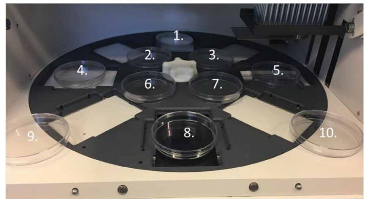
Figure 23. Example of LB plate layout within the KingFisher Apex instrument for 30 min decontamination protocol.
