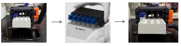
Semi-automated-lift 24 tubes simultaneously and then centrifuge-option 2
