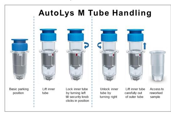
FFPE samples (curls, slides, cores) are placed in the tubes and protease digestion happens directly in them. After digestion is complete, the tubes are lifted from parking to the centrifuge position. Samples are spun allowing a physical separation of wax and tissue. Tubes are lifted to a final position so the lysate can be accessible for purification.
