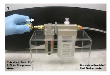
1. Insert the female quick disconnector fitting on the end of the 1/4" hose to the air inlet connector on the dryer unit.
