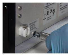
Insert the quick disconnector fitting on the end of the flexible tube (¼" OD, 1/8" ID) to the air inlet connector at the back of the instrument.
