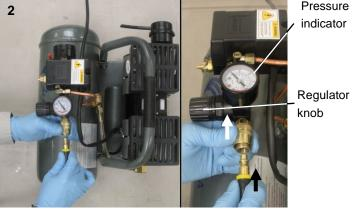
Insert the female quick disconnector fitting on the end of the ¼" hose to the air inlet connector on the dryer unit.
