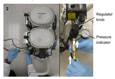
2. Connect the male quick disconnector fitting of the ¼" hose to the air compressor.
