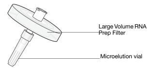
Figure 4-2 Filter-vial assembly
