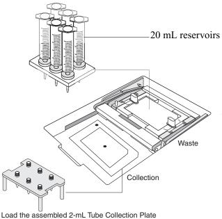
Load the assembled 2-mL Tube Collection Plate right before moving the carriage over to the collection position.
