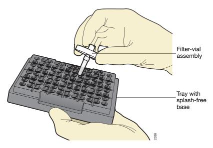
Figure 4-3 Filter-vial-base assembly
