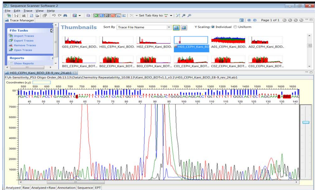
Figure 5 Severe dye blobs in the 60–65bp and 125–140bp regions
